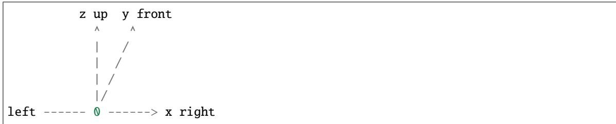
The definition of coordinate systems in this tutorial is actually **more than just defining the three axes**. For a box in the form of  $(x, y, z, dx, dy, dz, r)$ , our coordinate systems also define how to interpret the box dimensions  $(dx, dy, dz)$  and the yaw angle  $r$ .
